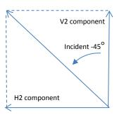
The magnitudes of the V1, H1 and V2 and H2 signals are all equal. Since V1 and V2 are the same, and H1 and H2 are the same, it appears as measured at the individual ports that the two incident polarisations have completely interfered with each other. For example, the overall cross polarisation isolation is 0 dB. This is in contrast to the case when the antennas of the same polarisation are used at both ends of the link where typically cross polarisation isolations of > 12 dB are achieved.
