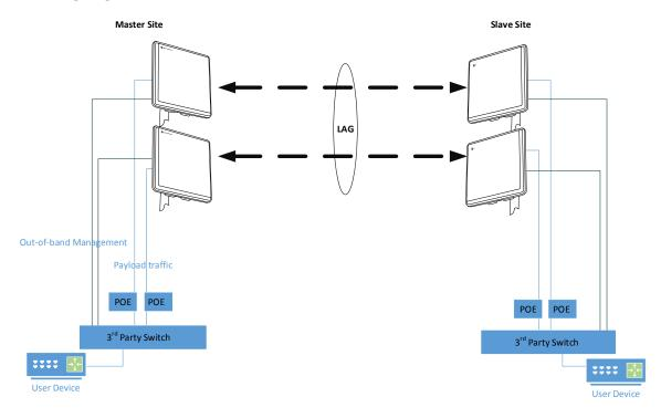
There will be two individual PTP650 1+0 links operating at the same time (PTP sync may be required depending on link planning because you are running two links at the same location at the same time). They are all connected to the same switch pair.
