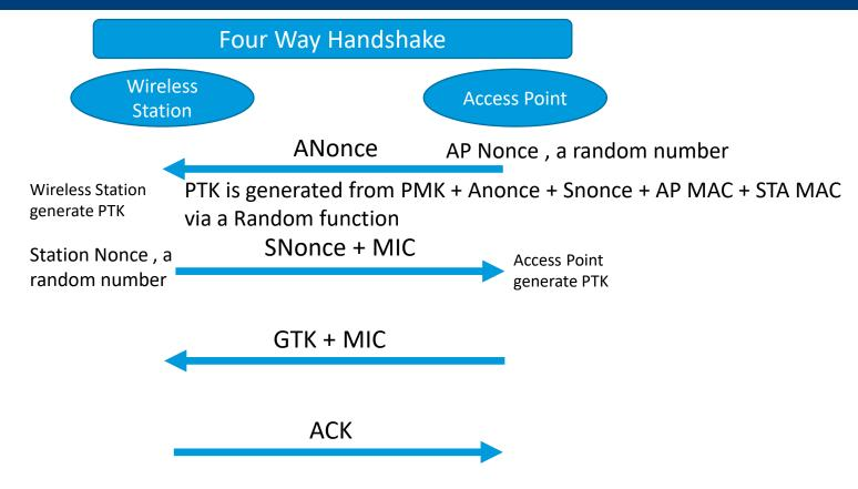
Four way handshake is used to generate PTK (Pairwise Transient Key) and GTK (GroupWise Transient Key). PTK is used for encrypting unicast wireless data packets.
