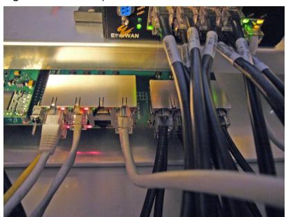
Figure 74 Staggered Ethernet cables
