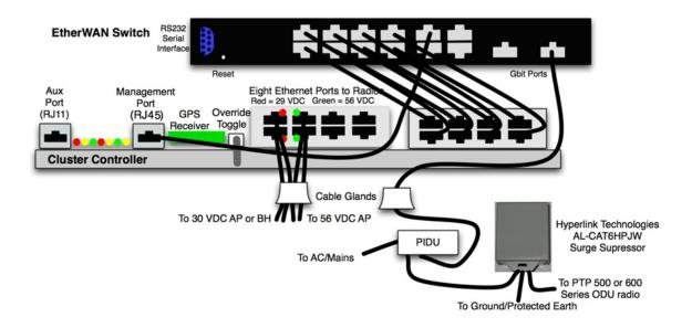
PTP 400 Series bridges operate at less than 100 Mbit speeds and so can be cabled to one of the eight Ethernet ports on the controller board, thus taking advantage of the controller board for surge suppression. The port must be configured to be unpowered. The PTP 400 Series bridge is powered by its own externally located PIDU.
