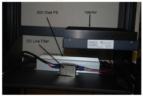
Figure 30: 600 Watt Power Supply Installation (rear view)
