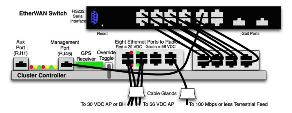
Figure 40 Rackmount CMM4 Standard Configuration
