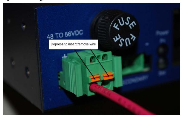
Figure 35: Wiring the Power Connector
