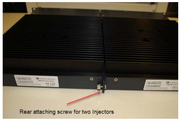
Figure 27: Rear Attaching Screw
