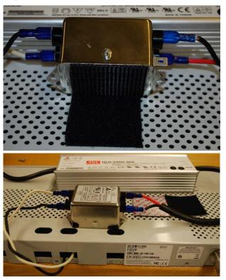
Figure 68 Rackmount CMM line filter installation (EU only)
