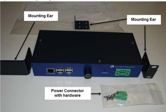
Figure 23 Installing a Single Controller
