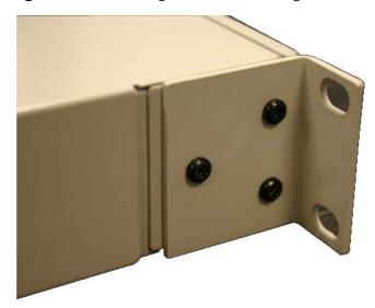
3 Select a 19" rack space in which the CMM4 may be mounted and use the (4) provided Phillips head screws to attach the front of the CMM4 to the rack
