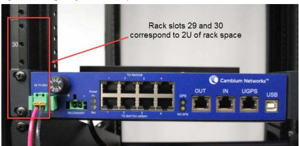
Figure 24: Single Injector Rack Space
