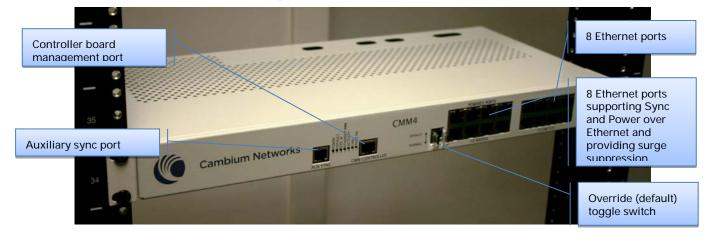
Outside the enclosure the CMM4 requires a GPS antenna and a power supply.
