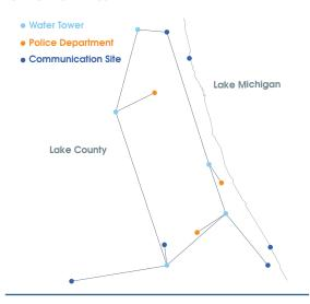
Above: ESRN replaced their leased lines with 4 and 2 wire cards. They integrated PTP 650 radios, a 4.9 GHz public safety network, and an OSPF network.
