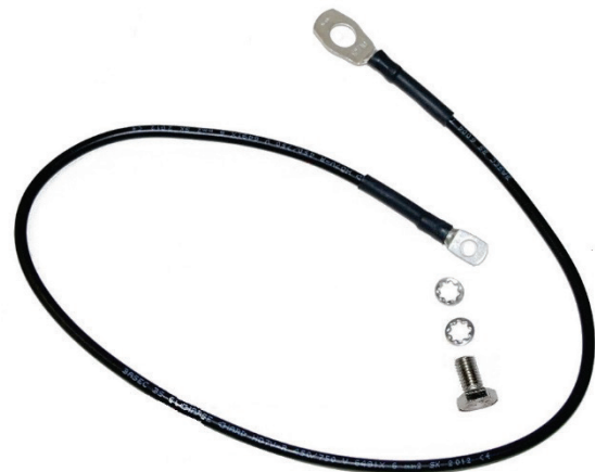
ODU to grounding system ground cable (M6 and M10 lugs), bolt and washers
