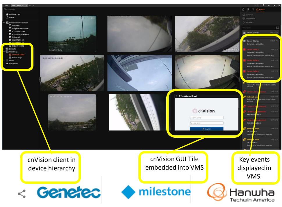
Single pane-of-glass monitor with VMS systems. Event based triggers from radio displayed on VMS. Basic parameters such as device up/down
