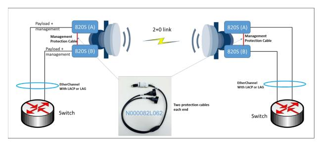
To enable "Mate Management Access", telnet to the radio's management interface. Run the following command (this will cause radio reset) on each radio,
