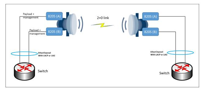
In this setup, the user configures one PIPE service on each 820S 1+0 link. The payload Ethernet port and radio port are also configured as a management service points to allow Inband management. The switch will run Etherchannel protocol (LACP/LAG) to aggregate the user traffic.
